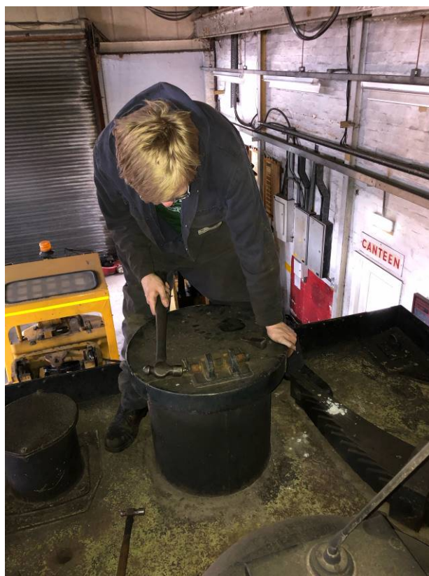
Jack Sharpe removing the pin in order to liberate the water filler lid. The lid/hinge assembly has been salvaged and will eventually be restored to the new tender tank.
