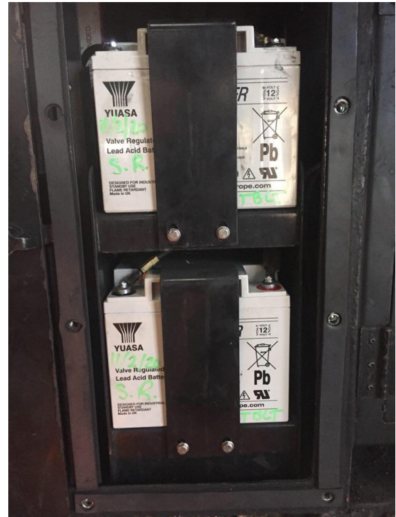
The new GSM-R batteries fitted in the tender battery compartment.
