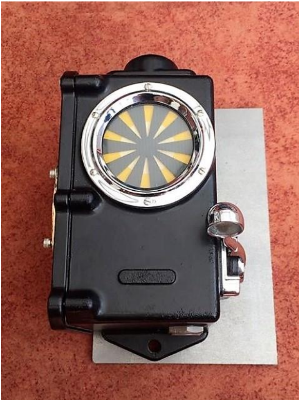
The overhauled 'sunflower' box roughly positioned on the newly made cab mounting bracket.
