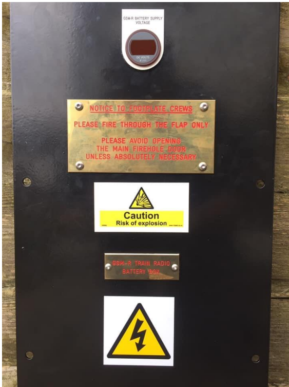
The GSM-R battery box cover after powder coating and fitting of the voltmeter.
