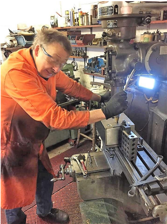
Steve Andrews is seen carefully drilling the holes for mounting the transducers in the box. This was done on his milling machine with the box securely clamped to the table of the machine. This allowed the holes to be drilled with considerable accuracy in comparison to using a pillar drill
