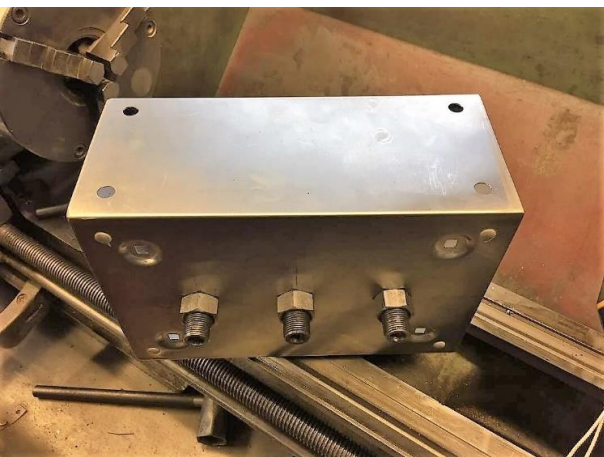
Externally the finished box with all the relevant mounting holes drilled and sharp edges removed. The work was undertaken in Steve Andrews' workshop because everything was conveniently on hand and an inordinate time was not spent searching for the right tools
