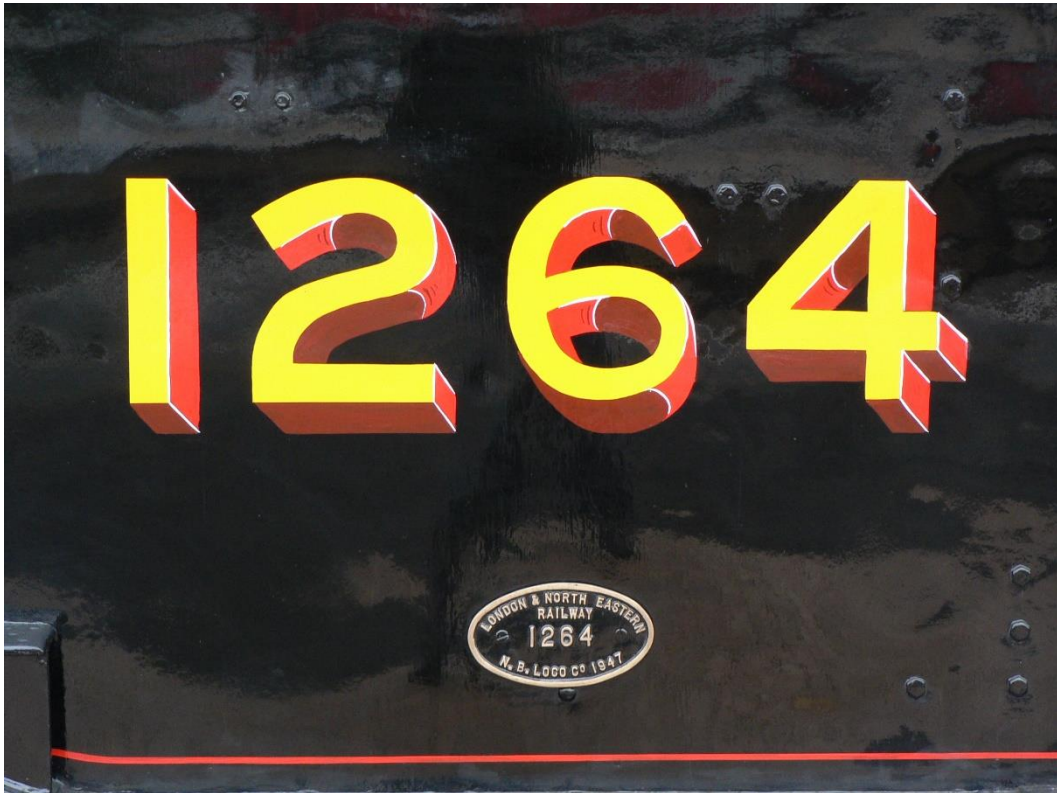
The completed cabside numbers finished in their red shading Photo courtesy of Alf Bousie
