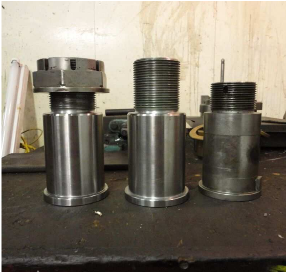
Some of the newly manufactured joint pins for the loco side rods.
