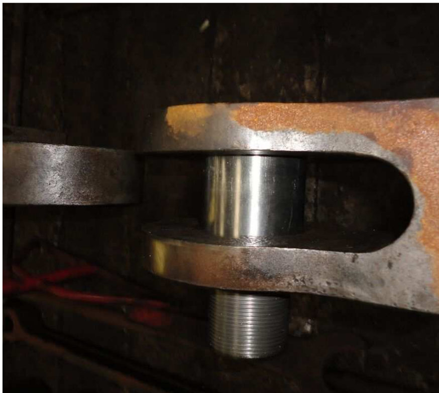
Test fitting one of the new joint pins into the fork of the coupling rod.
