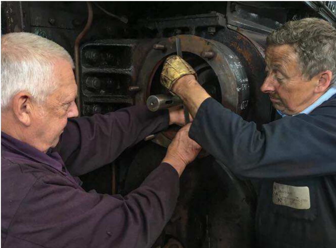
Keith Pardey (L) and Steve Andrews (R) take measurements of the left hand valve head so that the valve timing can be adjusted. Photo courtesy of Adrian Dennis.
