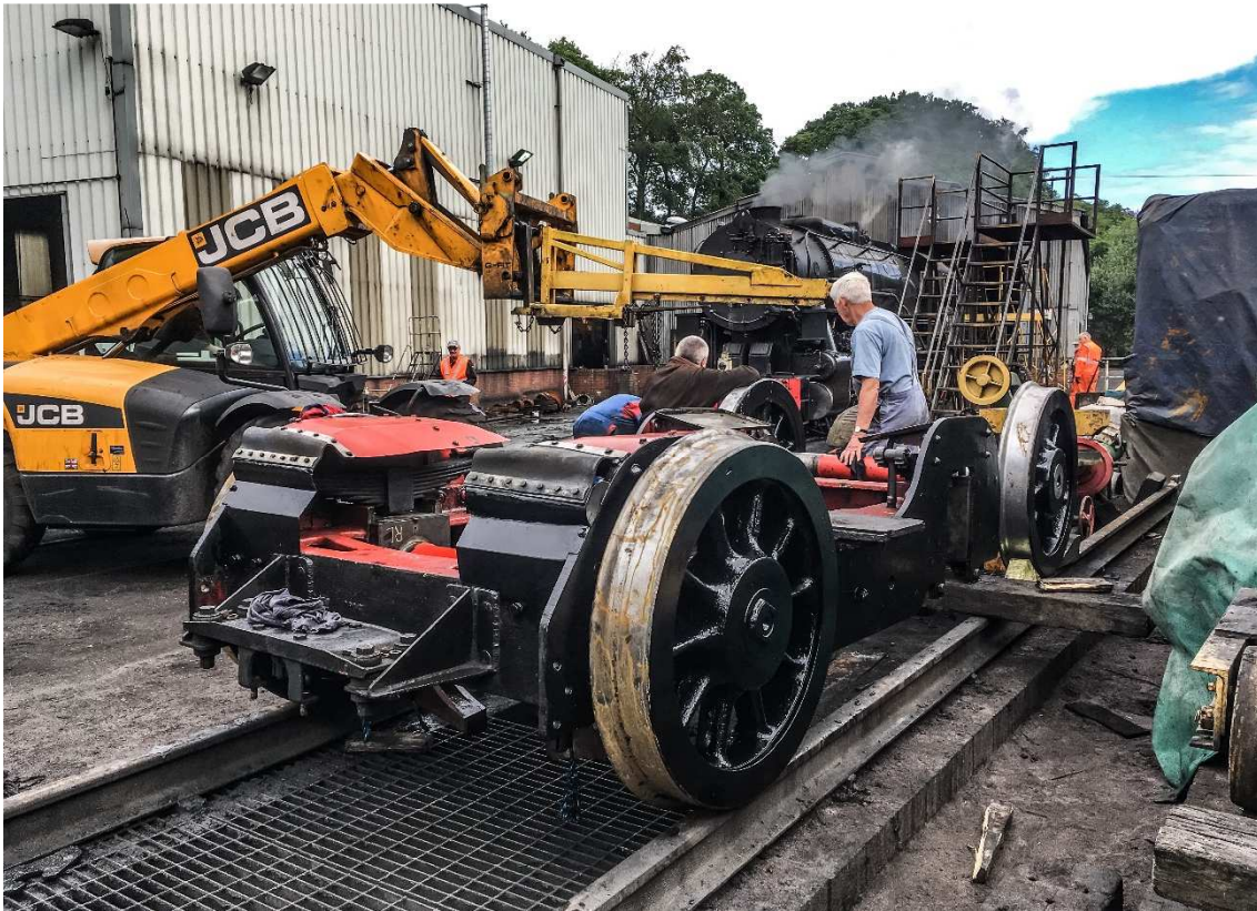
Steve Andrews along with Dougie and Duncan reassembling the bogie on 13 th July. Photo courtesy of Adrian Dennis / Grosmont MPD.
