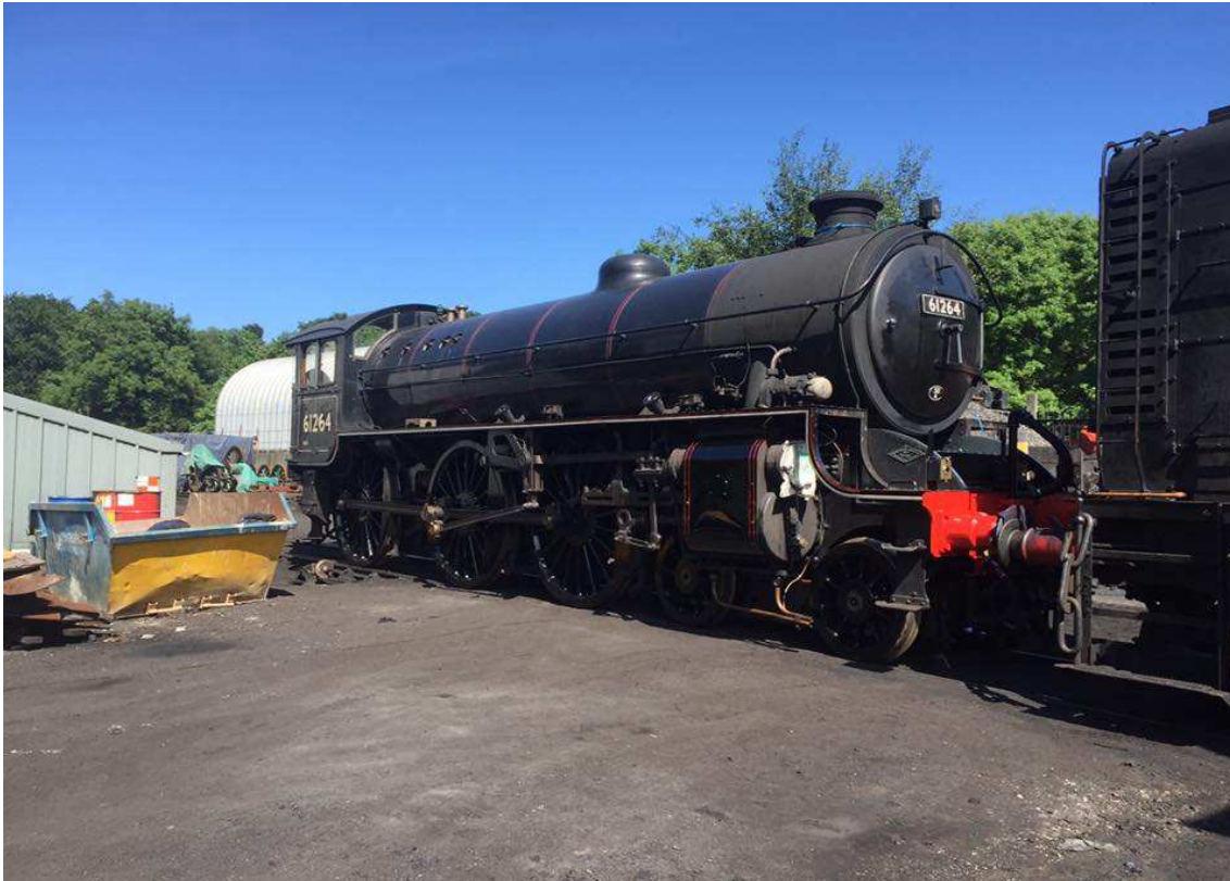
With the bogie back in place 61264 returns to being a 4-6-0 once again and waits to be shunted into the running shed to complete the remaining works. Photo courtesy of Mark O'Brien.
