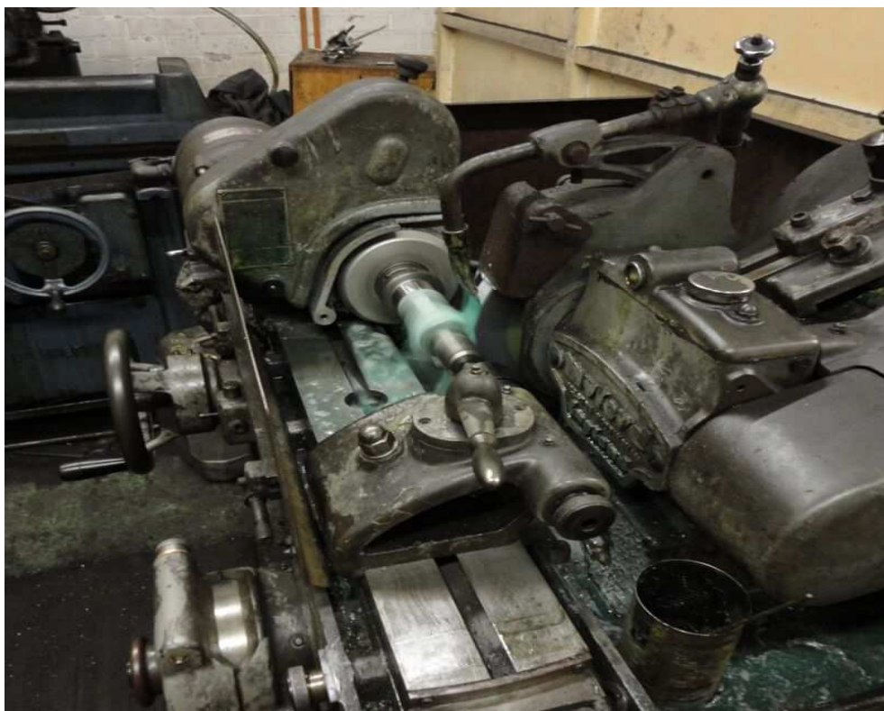
The pins mounted in a cylindrical grinder which by removing only small amounts of material with each pass ensures a perfectly even surface finish.
