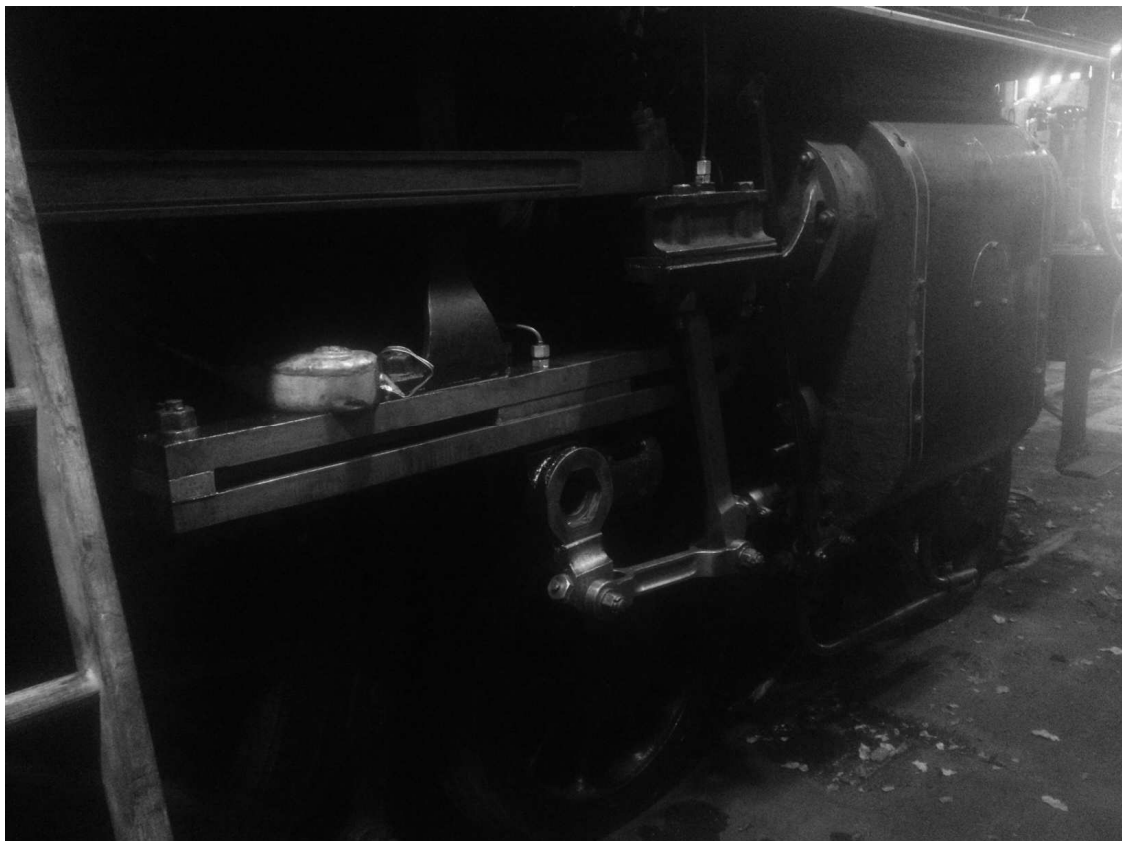
The motion with the connecting rod removed. Photo courtesy of Mark O'Brien.
