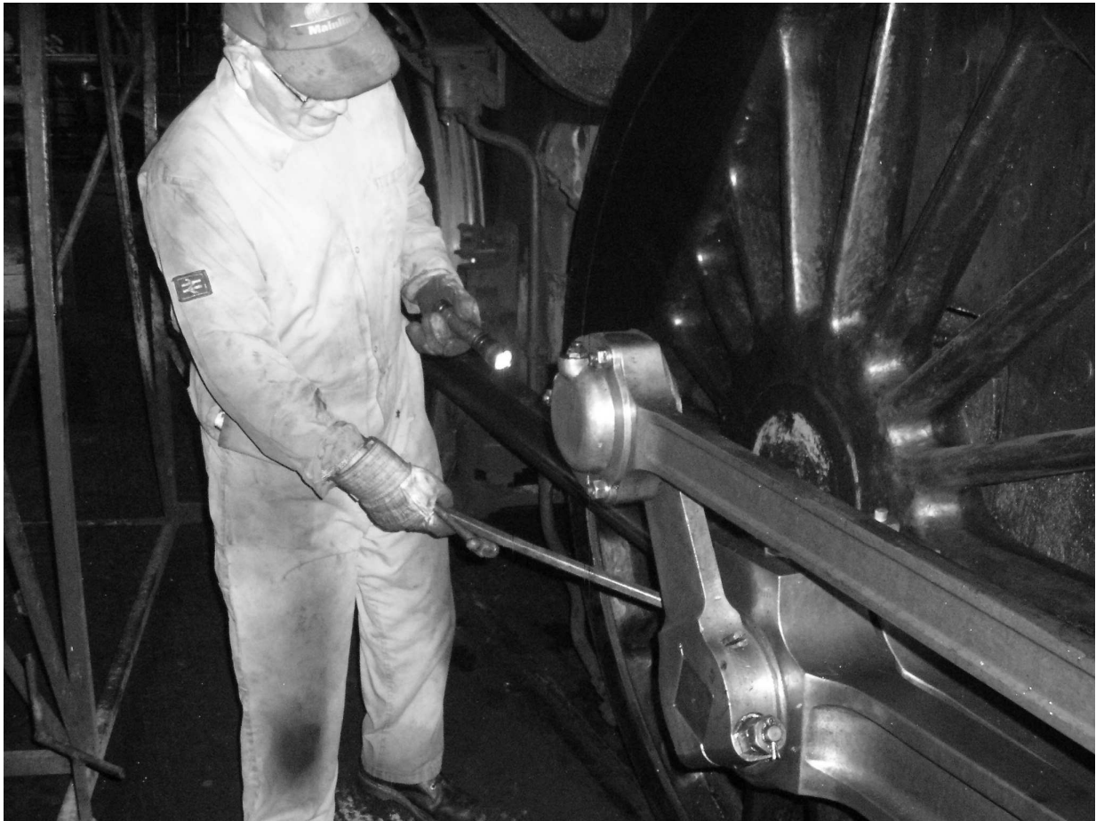
Chris Pinion checks for wear on the motion. Photo courtesy of Dave Fowler.
