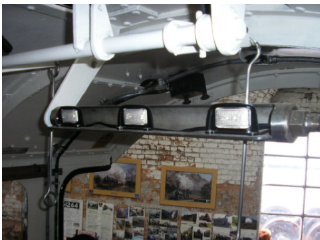
LED lights now adorn the freshly-painted cab – lighting up the backhead controls and gauges (left) and the footplate (right), not to mention the speedo and the injectors...
