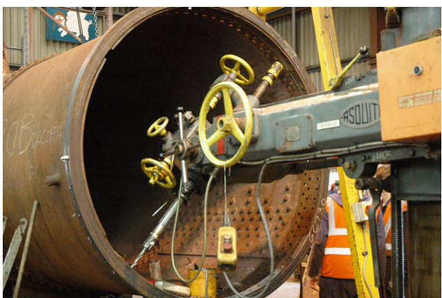
Work progresses at LNWR Crewe to drill the smokebox ring (left), using the old ring as a template. Meanwhile (right), bending the corners around the foundation ring, prior to drilling, reaming, tapping and riveting, is no easy job.
