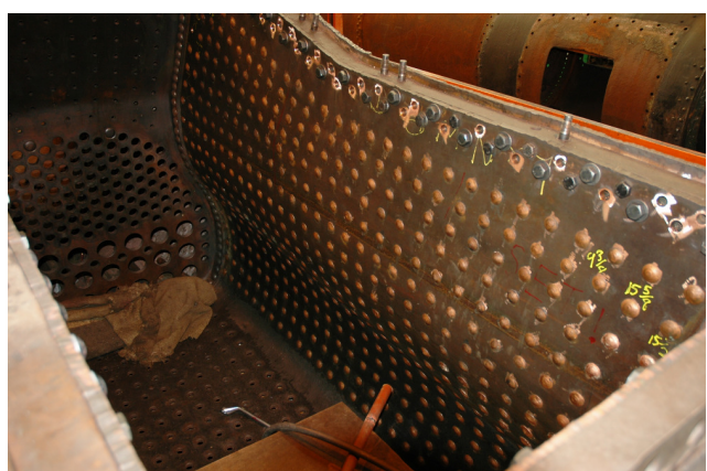
Much of the staying in the firebox is now complete (left), but we are still missing a pair of cab windows (right) – does anybody know of their whereabouts? If so please call Steve Andrews (07824 422029) or Mike Cobley (07803 073584).
