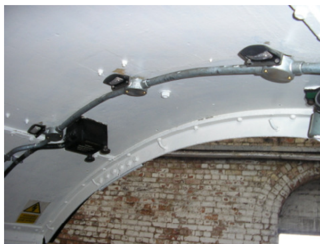
LED lights now adorn the freshly-painted cab – lighting up the backhead controls and gauges (left) and the footplate (right), not to mention the speedo and the injectors...
