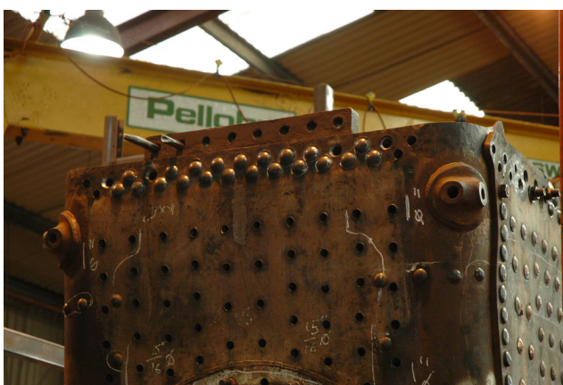
Work progresses at LNWR Crewe to drill the smokebox ring (left), using the old ring as a template. Meanwhile (right), bending the corners around the foundation ring, prior to drilling, reaming, tapping and riveting, is no easy job.
