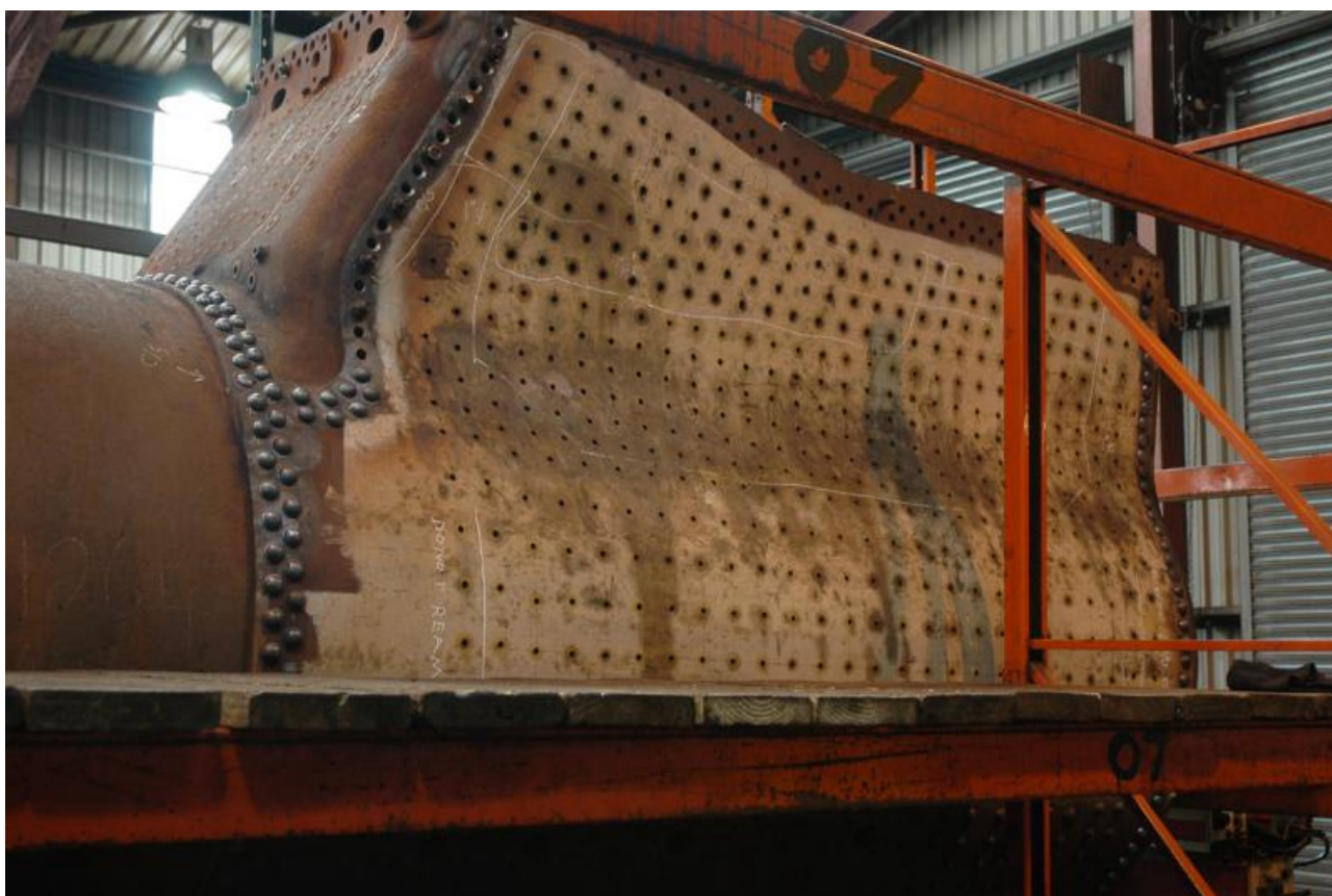
The outer wrapper and throatplate shown riveted to the boiler barrel. Note the chalk marks on the outer wrapper – these denote areas of same-sized stays. The holes are shown rough drilled, though most of the reaming is now complete.
