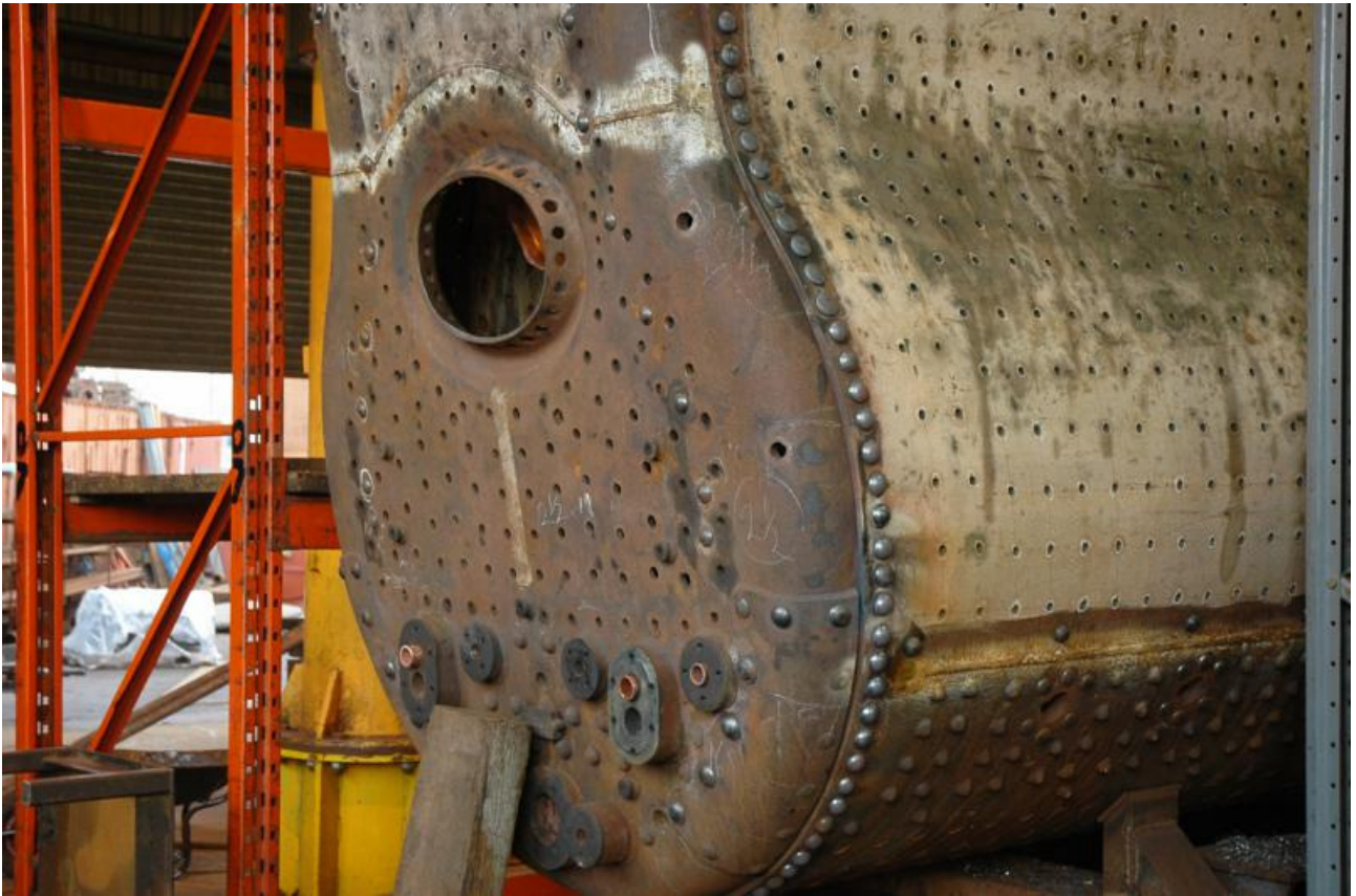
The doorplate, showing internal copper pipes protruding up to where the valves will be.
