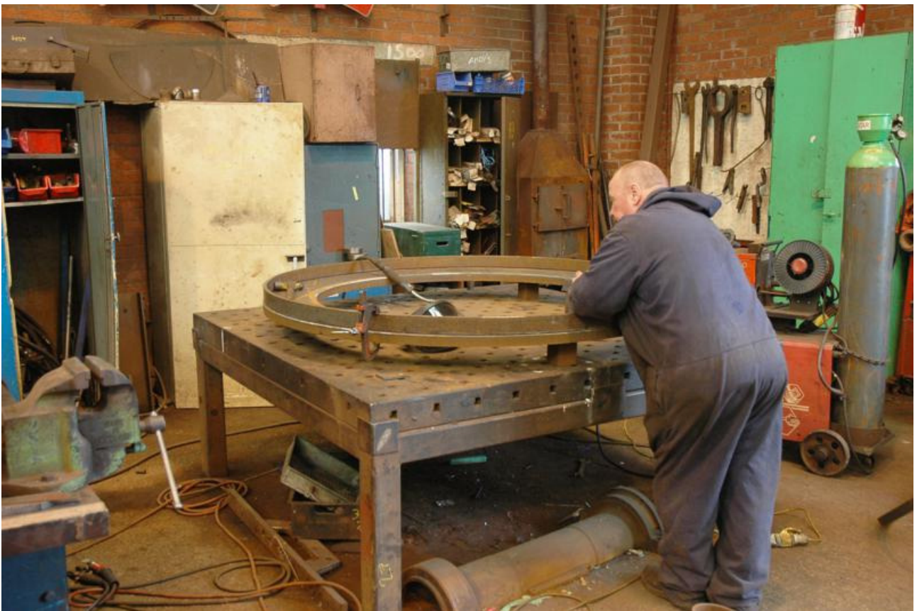
A start has been made on fabrication of the smokebox door ring.
