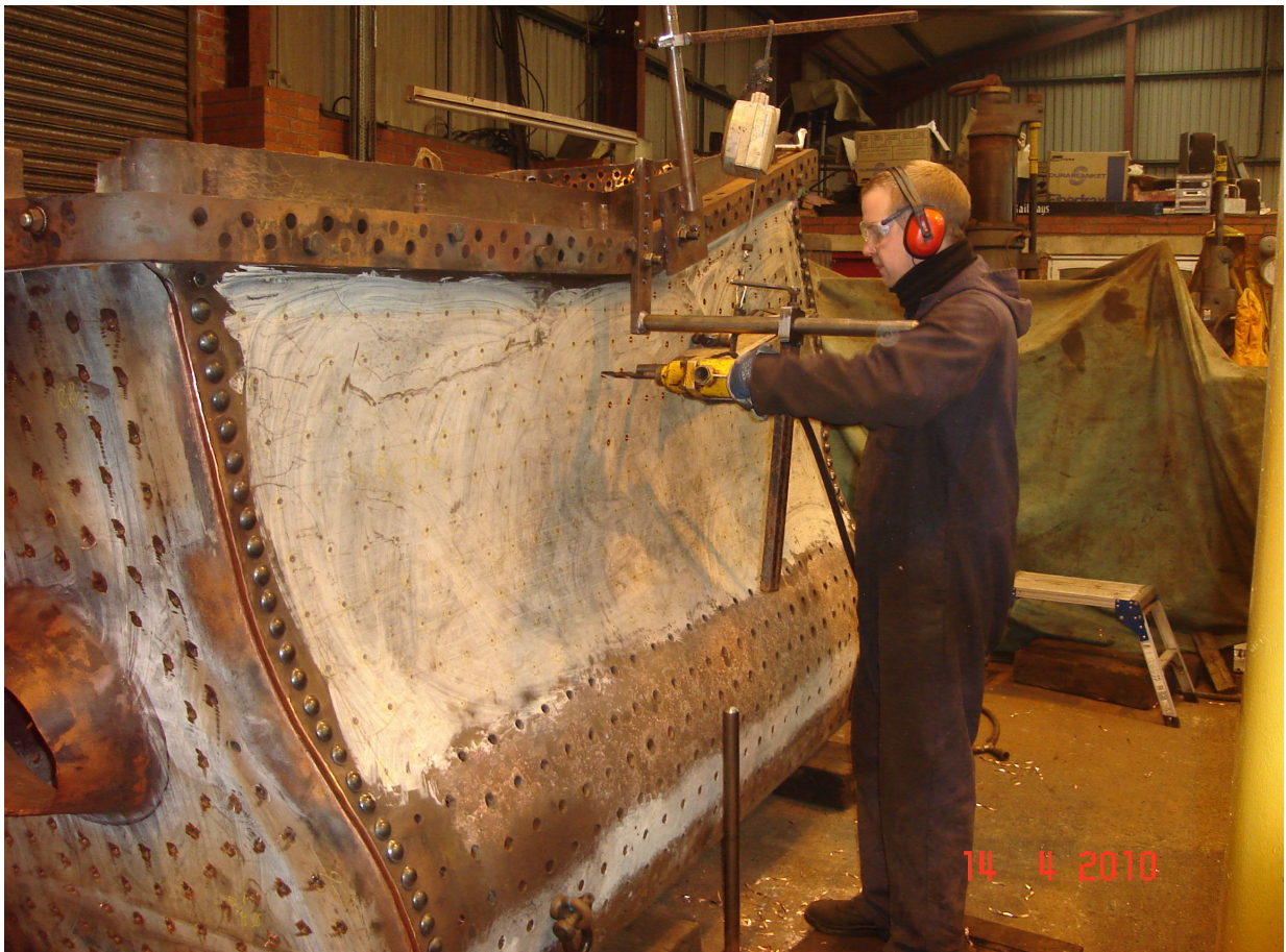
Copper firebox being drilled for stays.
