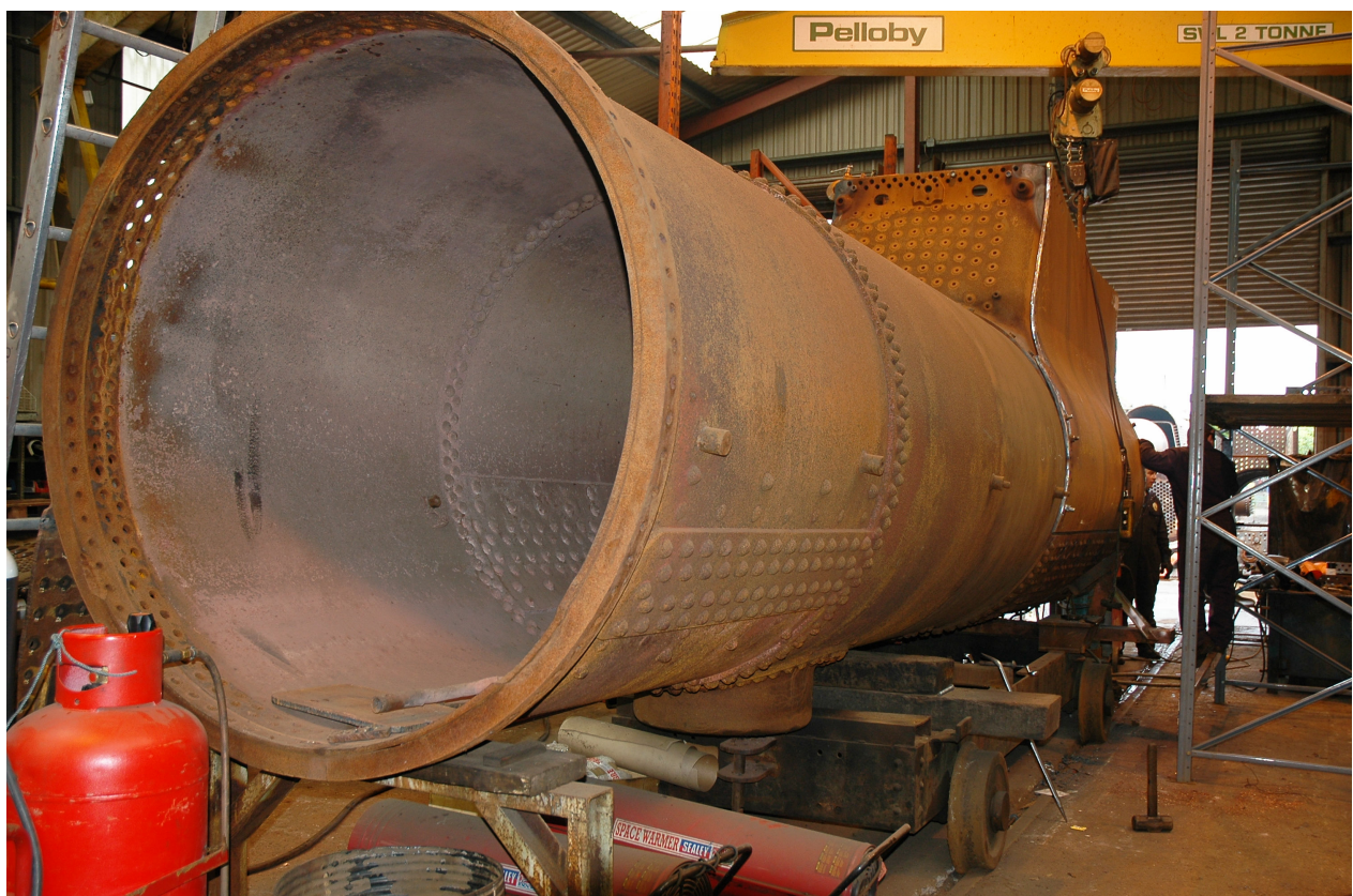
Trial fitting of the steel doorplate and steel side sheets. After this comes more drilling and then the insertion of the firebox, prior to the start of the final build and staying.
