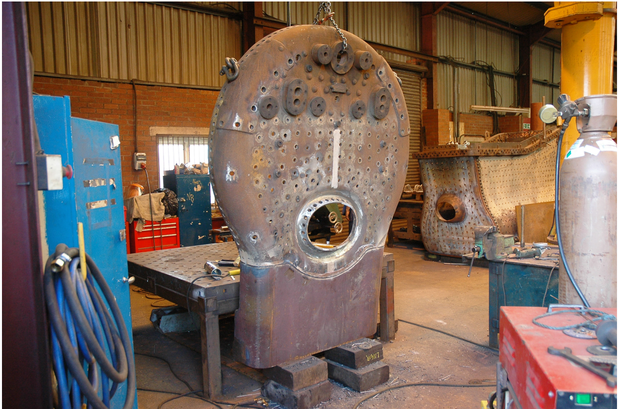
The existing upper doorplate and new bottom section are welded back together again.
