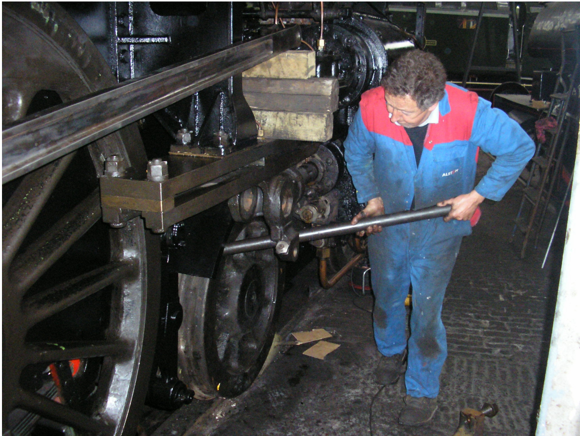
Steve Andrews gently eases back the off-side crosshead after splitting it from the piston.
