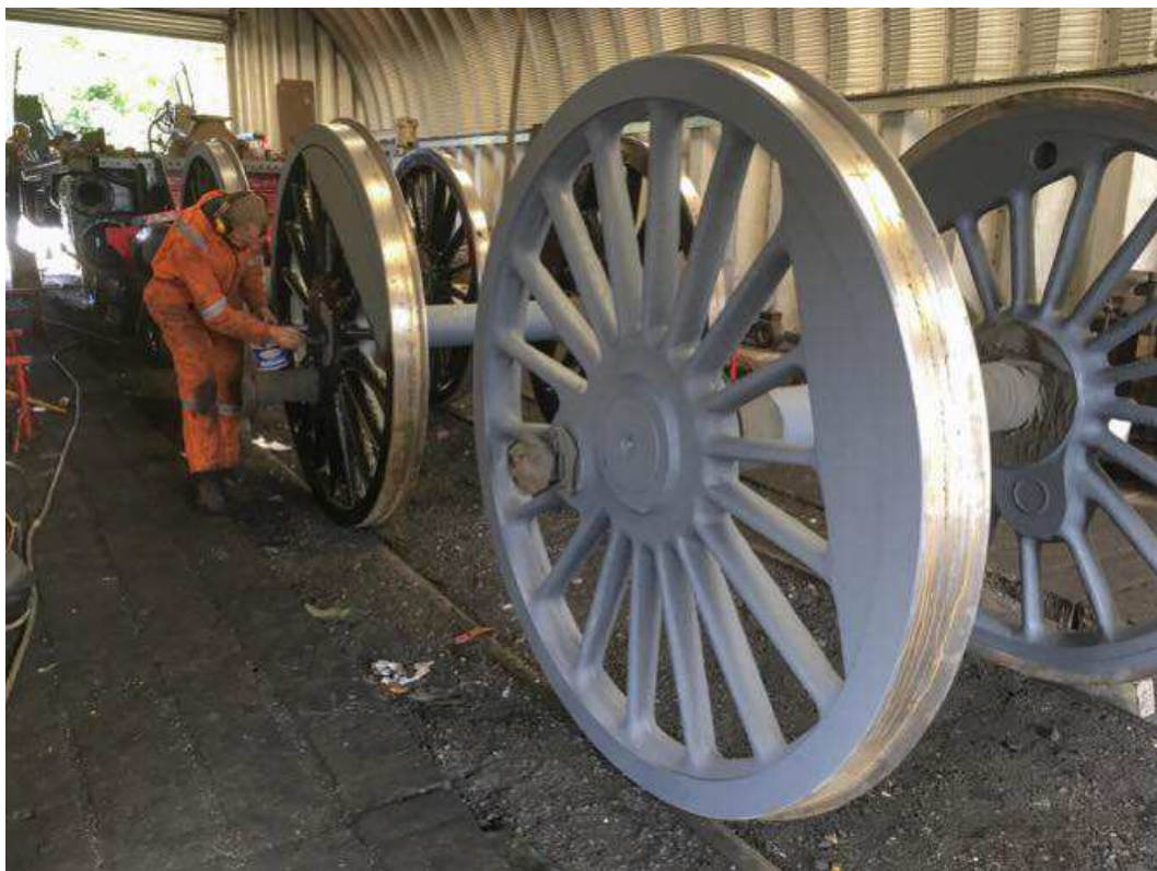
With preparation works completed John Furness commences painting. Photo courtesy A. Dennis / Grosmont MPD.
