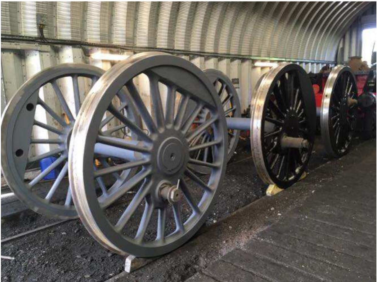
A very welcome sight indeed showing the fully repaired wheelsets back from Ian Riley & Sons and in the process of being painted. Photo courtesy of A.Dennis / Grosmont MPD.
