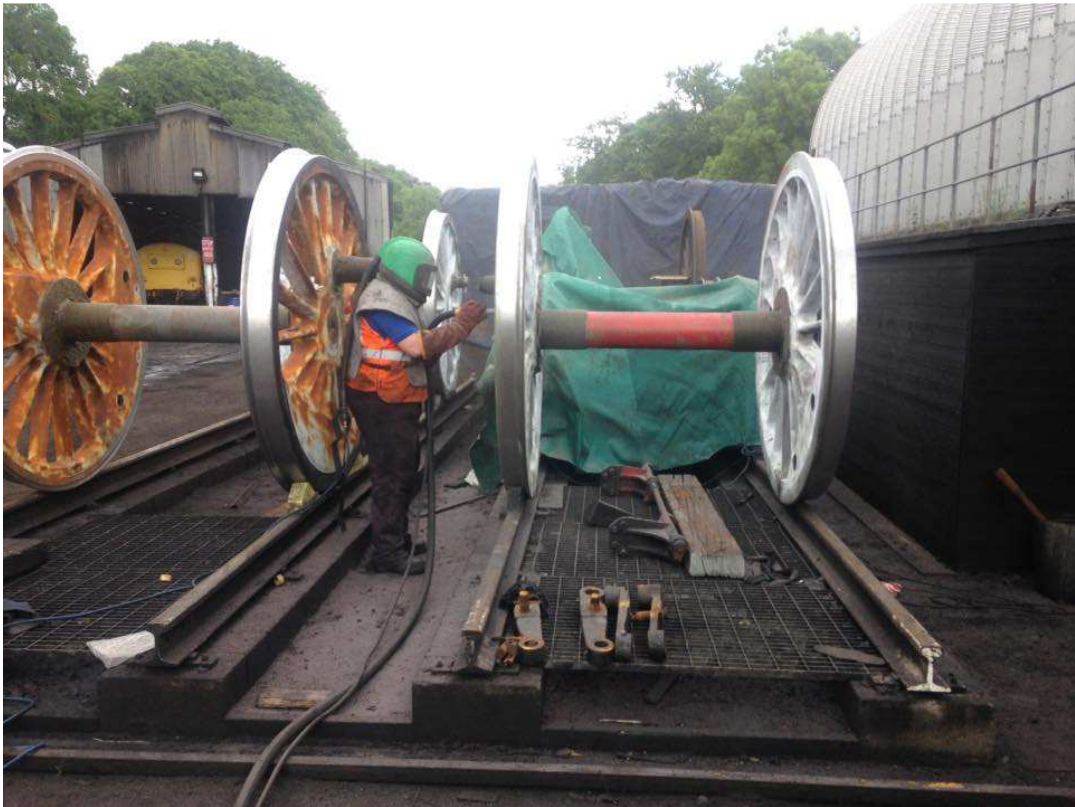
Adrian Dennis starts shotblasting the wheels to remove any rust and residual paint. Photo courtesy A. Dennis / Grosmont MPD.
