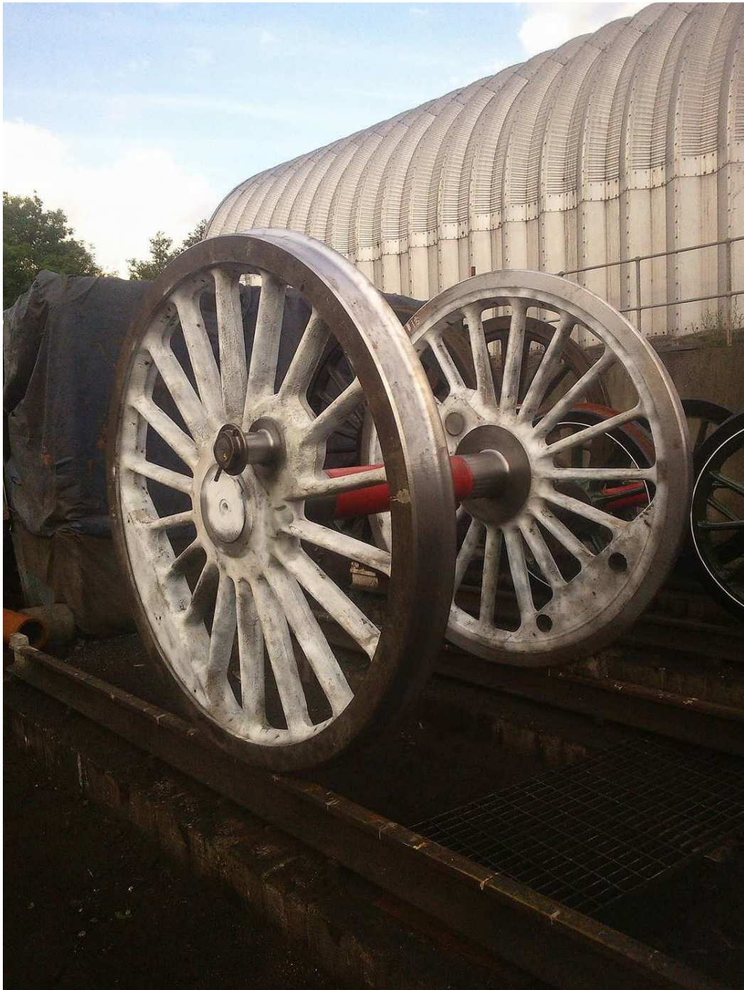
When the wheelsets were returned to Grosmont they were still covered in the white dye penetrant spray, used to check for cracks.
