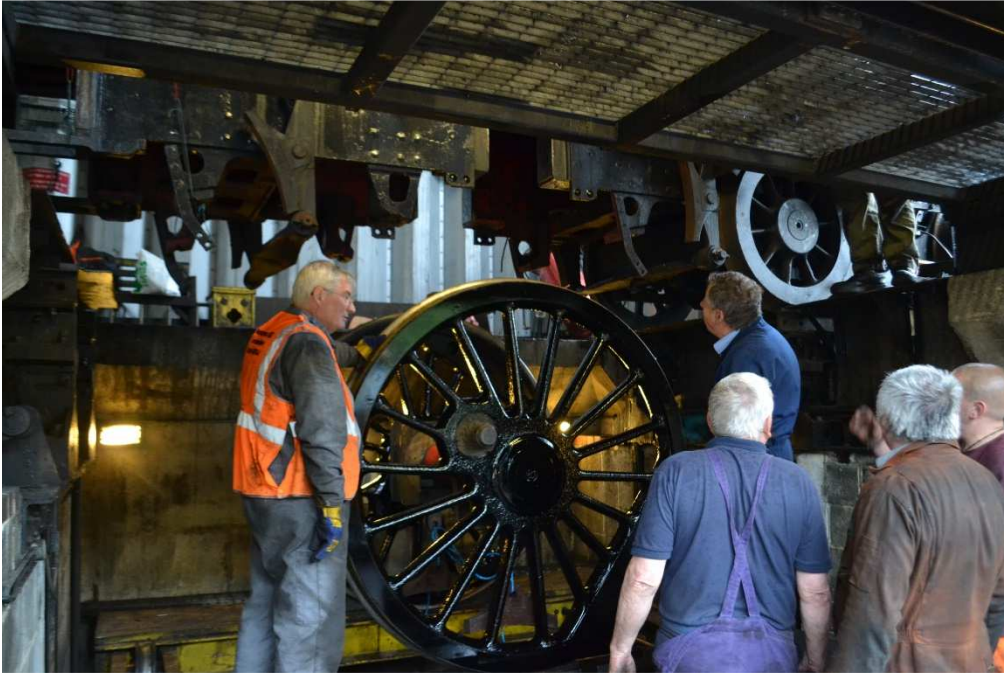
An audience watches with anticipation as the leading wheelset is prepared for installation on the Grosmont wheel (ex-Hull Dairycoates depot). Photo courtesy of Dave Wellington.
