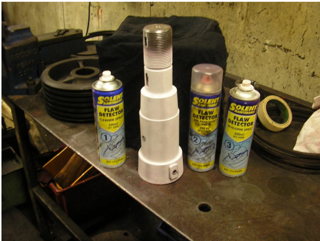
The magnetic particle inspection of the little end pin. Photo courtesy of Dave Fowler.
