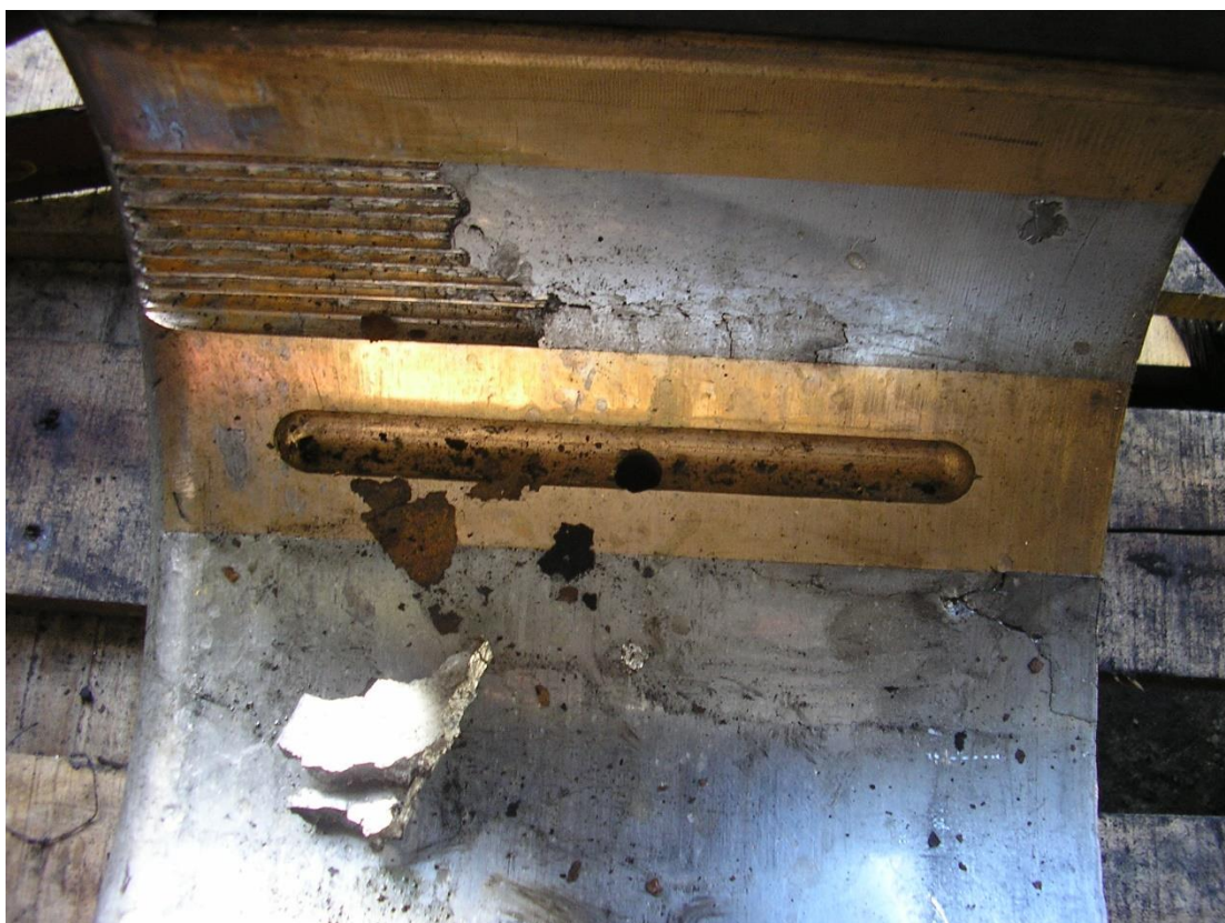
The damage to the axlebox showing the white metal broken up and dropping out of the serrations in the bronze crown. Photo courtesy of Dave Fowler.
