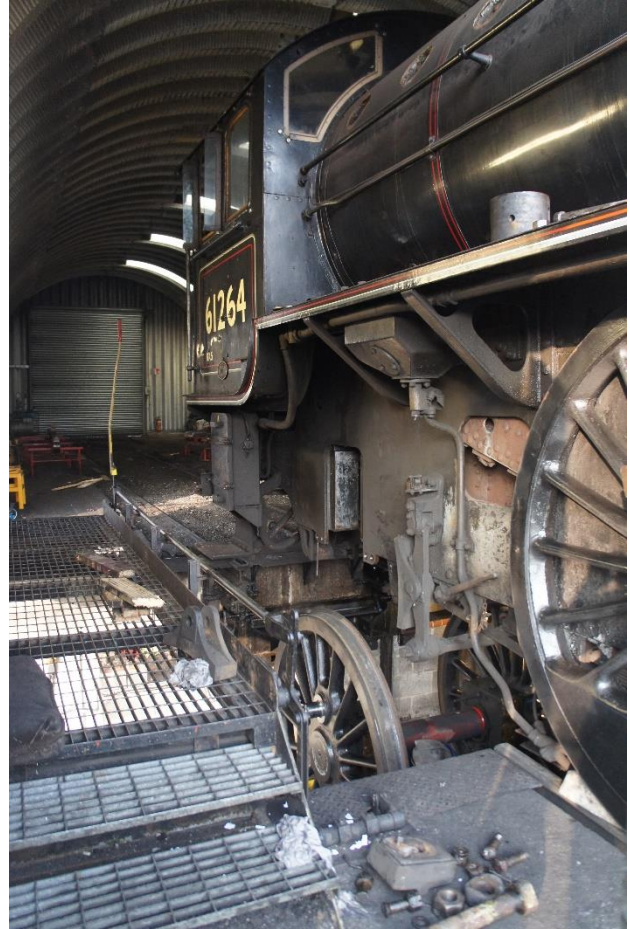
Left: the loco over the wheel drop having the trailing wheelset removed ready for the inspection of the axleboxes. Right: the rather unnerving sight of the loco perfectly balanced on the front bogie and remaining wheelsets. Both photos courtesy of Steve Robb.
