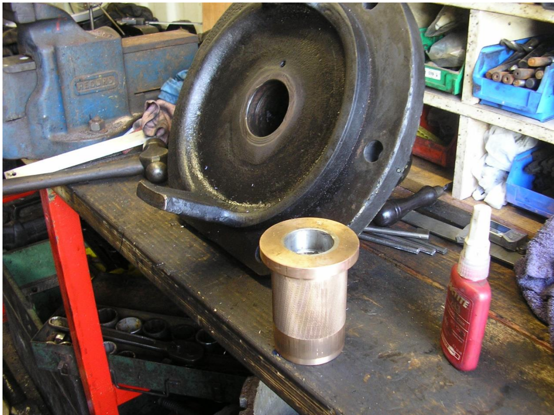
One of the bushes made by Steve Andrews for the valve spindle end cover. Photo courtesy of Dave Fowler.
