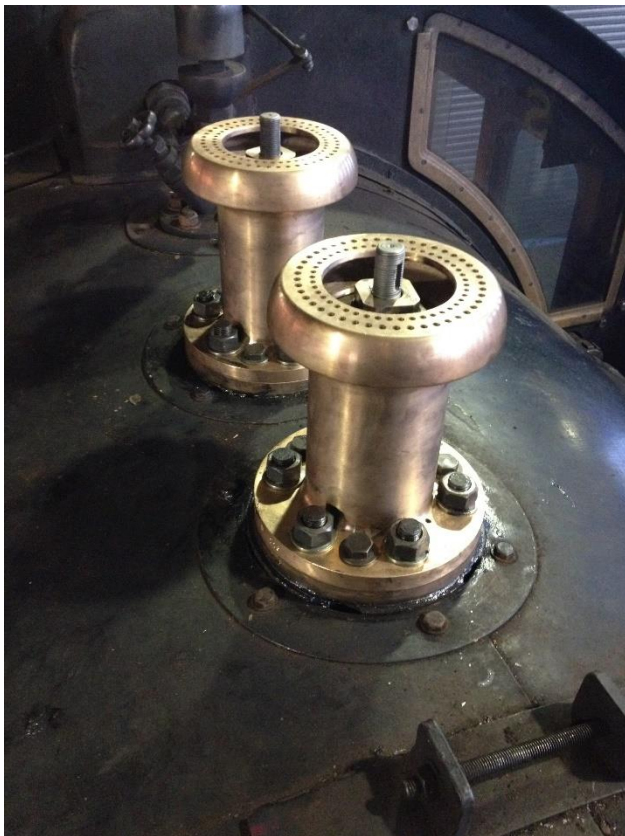
Left: The newly fitted safety valves mounted on the boiler ready for setting on steam pressure. Right: the boring gear is seen attached to the RHS cylinder during the process of boring it out to take a cylinder liner. Both photos courtesy of Steve Robb.
