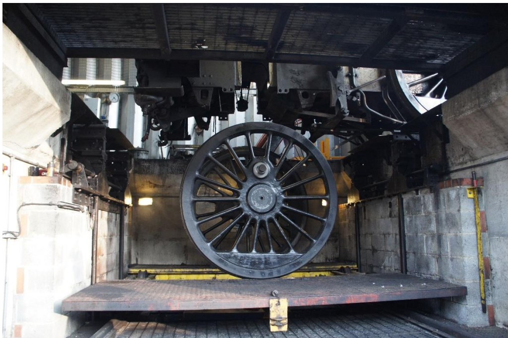
The trailing wheelset lowered to reveal the axleboxes. Photo courtesy of Steve Robb.
